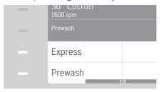
Select the desired option/s by pressing the light bar or the corresponding symbol. Selected options change colour and are shown in the upper part of the display.
