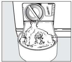
■ Unscrew the drain filter lid until water runs out.
