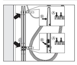
Secure the transit bars to the back of the machine. Make sure that holes ® are fitted over retainers A.
