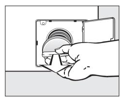
■ Remove the drain filter completely.
